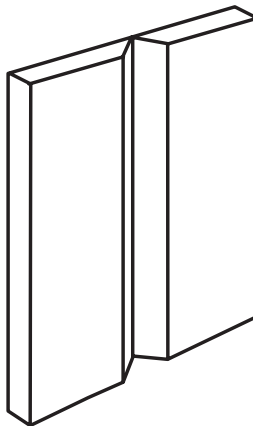
(C) VERTICAL WELDING TEST POSITION 3G
